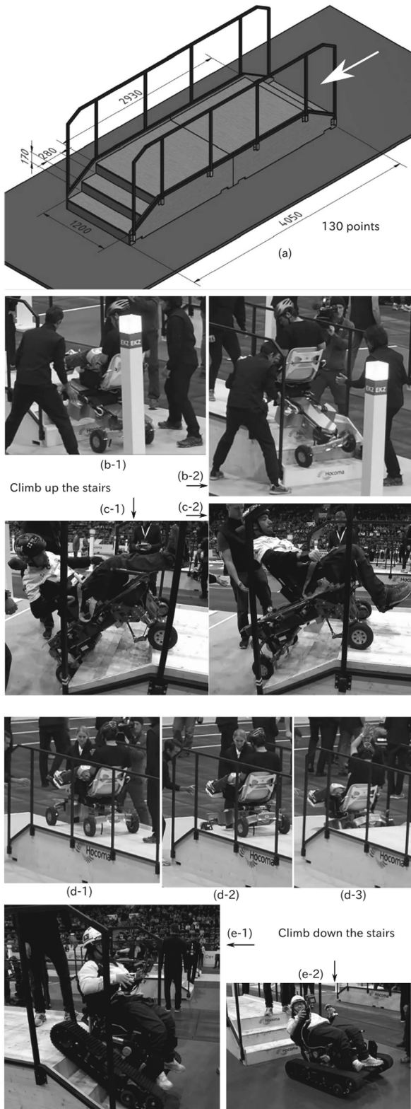
Fig. 12 Stairs task: (a) dimensions of the course, (b-1, b-2, c-1, c-2) scenes at climbing up the stairs, (d-1, d-2, d-3, e-1, e-2) scenes at climbing down the stairs ((a) is from the rule book and (c-1, c-2, e-1, e-2) are captured from videos by ETH Zurich/SRF)
